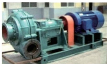
排泥泵 Peed and Discharge slurry pump
