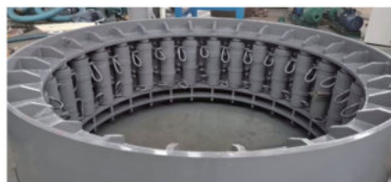
中继器 Intermediate Jacking Station
